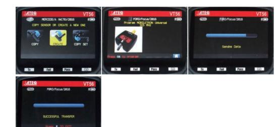
Select 'Copy' to copy/clone an existing TPMS sensor. When directed scan the existing TPMS sensor with the ATEQ tool.
